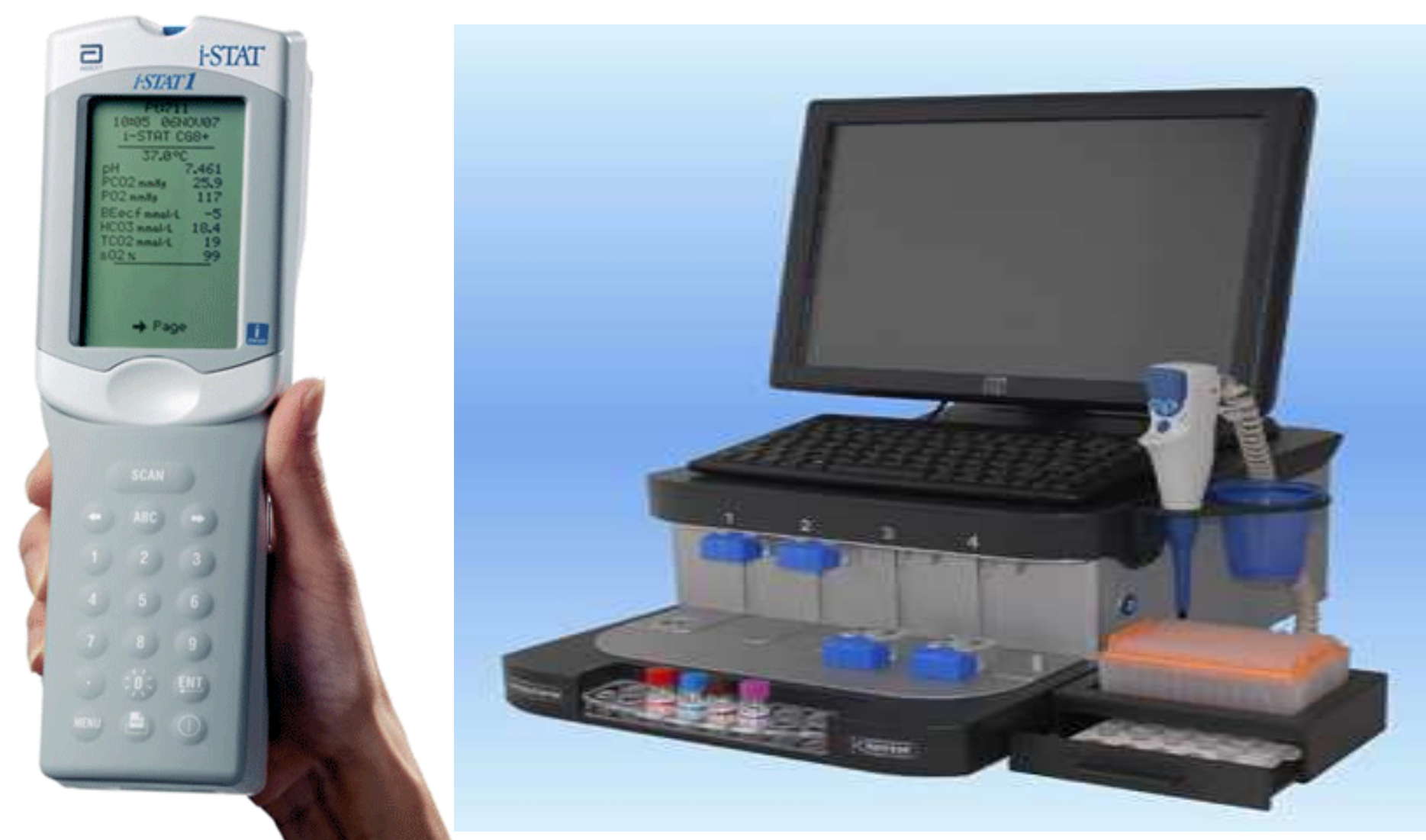
Figure 1: Point-of-care measurement devices: Measurement of hemoglobin/hematocrit was performed using the i-STAT ® handheld analyzer and i-STAT ® CG8+ test cartridges (Abbott Point of Care, Princeton, NJ), viscoelastic testing was performed using a ROTEM ® delta device (Tem Innovations GmbH, Munich, Germany)
